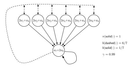
**Figure 11.1:** Baird's counterexample. The approximate state-value function for this Markov process is of the form shown by the linear expressions inside each state. The **solid** action usually results in the seventh state, and the **dashed** action usually results in one of the other six states, each with equal probability. The reward is always zero.
